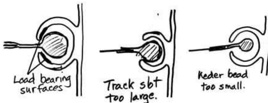
Designers and builders working with tracks have many choices. It is always appropriate to match material and design considerations with known loads and functions. For example, it is common to use 13mm (heavier) attached to tent top fabric but only 11mm attached to side panel fabric in the same size tracks. Overall, the system must retain and support the fabric as intended, withstanding load and stress forces without failure.
