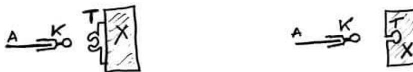
There is only one true defining function –connecting a sheet to a rail; a basic system of attachment. The intent is to connect a fabric sheet (A) to a solid rail (X). The system must include two parts, the keder itself (K) and a track (T) to hold it. Sometimes the track is built into the solid rail and other times it's added on. Therefore, the application can be either a four-part connection: A and K joins T and X; or a three-part connection: A + K joins to TX.
